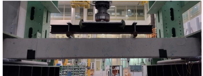
Four-point bending test under static loading<sup>5</sup>
