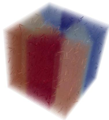
*Domain decomposition approach based on a geometric bisection for  $ID = 2$  with  $n^{proc} = 8$*
